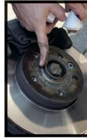
Apply a thin layer of corrosion protection paste to the centering flange on the spacer.
